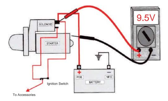
Crank the engine for about 10 seconds while observing the voltage reading. A reading of 9.5 volts or more would indicate there is sufficient voltage being supplied to the starter to operate properly. If the starter does not function like it should, chances are the starter is defective or the engine has a problem, causing it to be difficult to turn.
